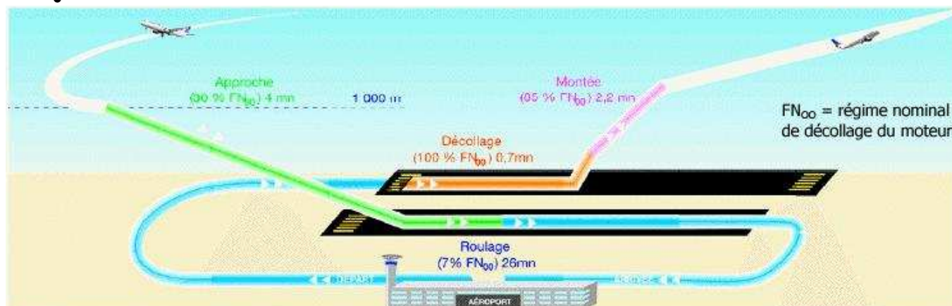
Figure 29: Phases du cycle LTO
